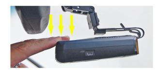
4 - If the RD is too close to the bottom of the mirror, You may access the buttons on top of the RD by gently pushing downward on the front of the RD with one finger and push the desired button with another finger. Then allow the RD to return to it's original position by gently letting it spring upward. When accessing the buttons, be sure to push the RD downward just enough for your finger to fit between the RD and mirror.
